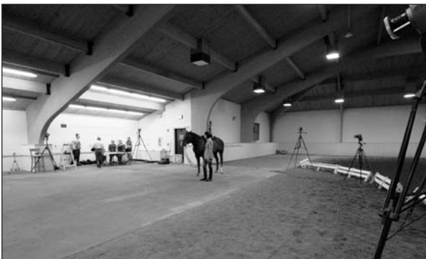
Fig. 5: View of the data collection runway and alcove in the Mary Anne McPhail Equine Performance Center at Michigan State University; the horse is standing on the force plates in the center of the data collection volume and several cameras are visible distributed around this volume. (Photo credit: Britt Larson)
