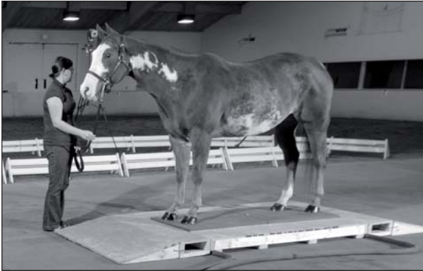
Fig. 3: Horse standing on a platform with embedded 2 force plates to measure the location and movements of the horse's center of pressure (Photo credit: Erin Grooms)
