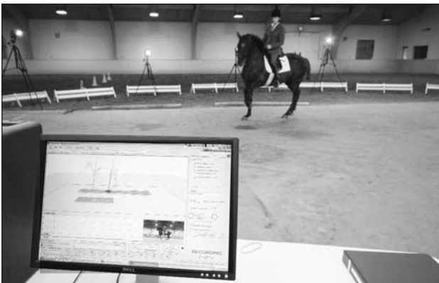
Fig. 4: Horse cantering over the force plate system in the Mary Anne McPhail Equine Performance Center at Michigan State University; the runway is viewed from behind the screen of the Motion Analysis System (Motion Analysis Corp., Santa Rosa, CA). The screen shows a real time image of the horse as a stick figure, including the corresponding ground reaction force vectors. 3 of the 10 infrared cameras arranged around the data collection volume. are visible behind the horse (Photo credit: Britt Larson)
